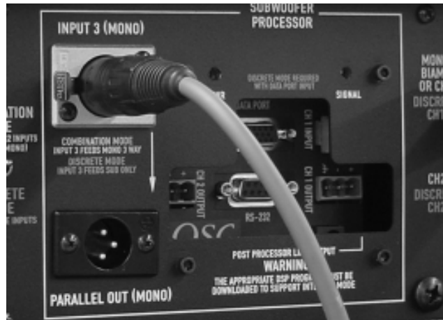
INPUT 3- In Combination Mode, Input 3 is used for mono 3-way input to both processors. In Discrete Mode, Input 3 is used for the subwoofer only.
